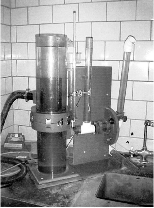
FIG. 1 Constant and Falling Head Permeability Apparatus
